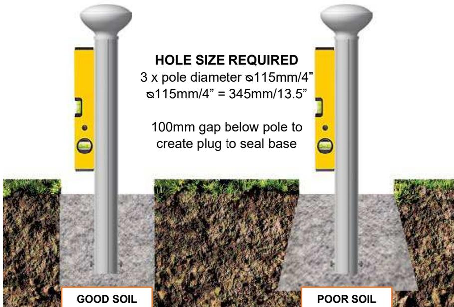
A **much larger foundation may be required** if soil is poor/sandy to prevent bollards being pushed over or removed/stolen. Try and taper out towards the bottom so the base section of concrete is larger than the top section as per this image
