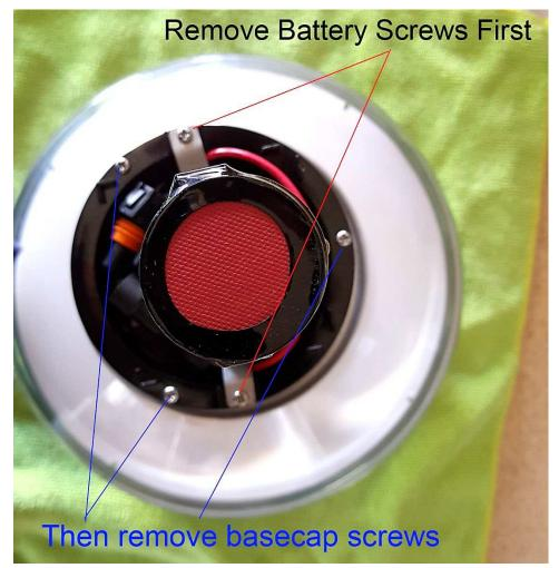
2. Slowly pull out the base cap from the base section without pulling on the solar panel cable to hard.
