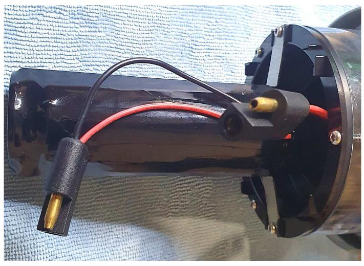
9. Connect the new weatherproof battery connectors together exactly as shown below to activate power to the unit.
